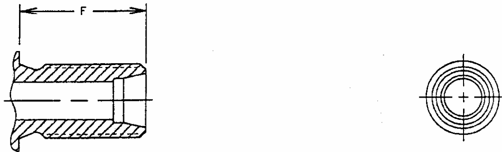
FIGURE 2 - FITTING END DESIGN, STYLE E SAME AS STYLE S EXCEPT AS SHOWN
